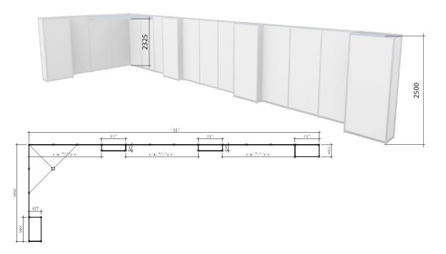
Partition walls between headstands must be constructed double-walled. Such a double wall should have a depth of at least 0.5 m. If supporting walls with a depth of 0.5 m are used this stand space is lost.
